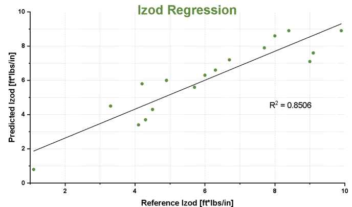
Fig. 4 shows a regression model developed for the prediction of Izod by lab IMR (MagStation II) for pellets. Its root mean square in this example is 0.85.
